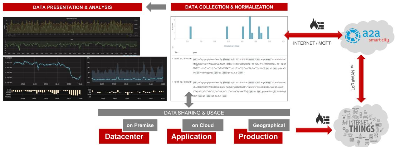
\*LoRaWAN™ is a Low Power Wide Area Network (LPWAN) specification intended for wireless battery operated Things in a regional, national or global network \*MQTT is an ISO standard (ISO/IEC PRF 20922) publish-subscribe-based "lightweight" messaging protocol for use on top of the TCP/IP protocol.
